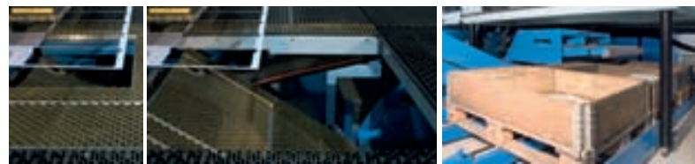
Two drop doors for laser cut parts Sorting of small pieces into sorting boxes
